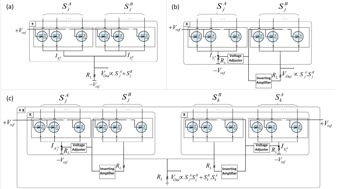
Figure 3. Segment-level Composers; (a) Addition SLC, current summation is used to perform addition; (b) Multiplication SLC, the current of one multiplicand is used to modulate the reference voltage of the other multiplicand, resulting in a multiplication operation; and (c) Add-Multiply SLC, a hierarchical combination of the addition and multiplication SLCs which implements a sum-of-products operation.
