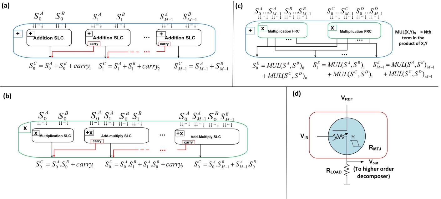
Figure 4. The Flat-Radix Composers; (a) Addition FRC made up of several addition SLCs and carry circuits; (b) Multiplication FRC made up of one multiplication SLC and several Add-Multiply SLCs and carry circuits; (c) Add-Multiply FRC made from a hierarchical combination of Multiplication FRC and Addition FRC; and (d) Carry propagation circuit providing carry support from lower order segment to higher order segment.
