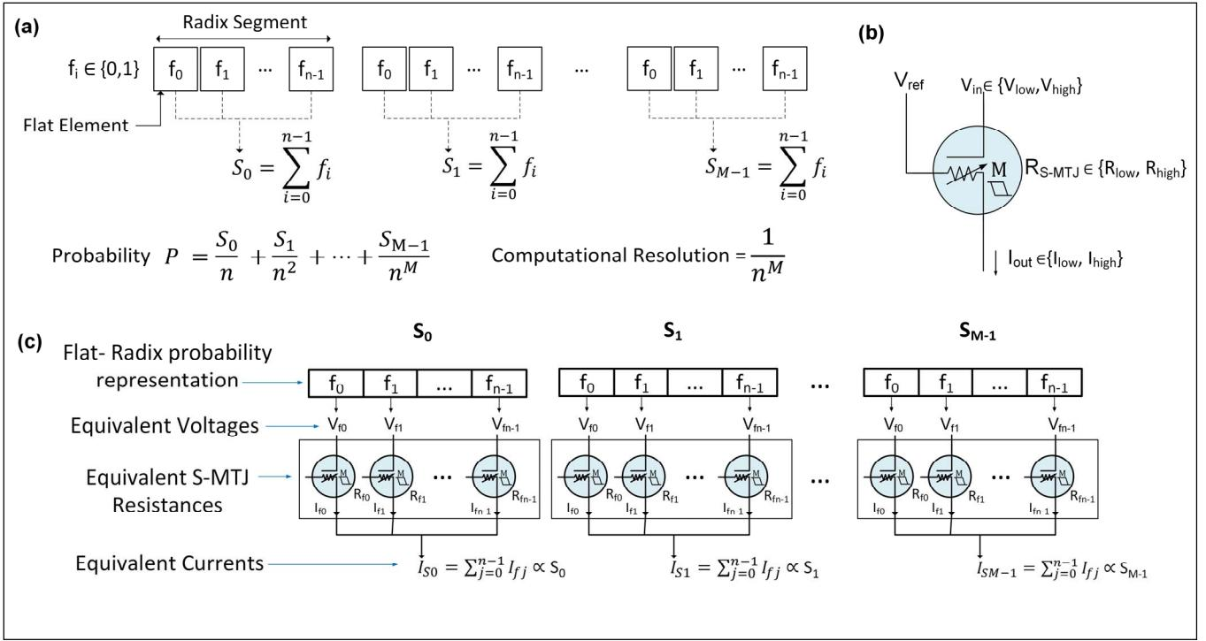
Figure 2. (a) Flat-Radix information representation scheme. Probability is encoded in segments which are in a radix arrangement, with each segment containing flat elements; (b) Schematic view of the 2-state S-MTJ device [12][13]; (c) Physically equivalent encoding of probability using the proposed information representation scheme.
