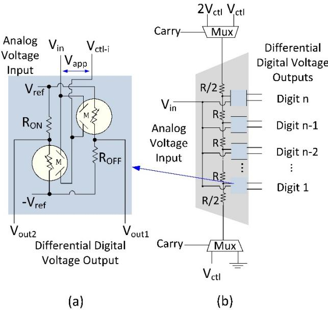
Figure 5. The decomposer circuit. (a) A single comparator element of a segment-level decomposer; and (b) A segment-level decomposer implemented by structuring individual comparators in a R-2R circuit.
